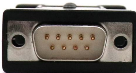
Figure 2.3 GCAN-403 converter fault-tolerant CAN interface form
