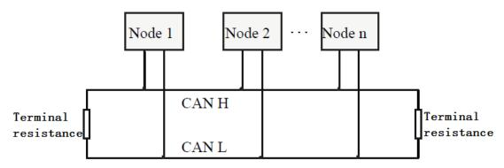
Figure 3.1 CAN-bus network
