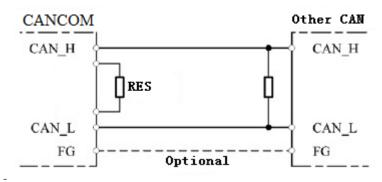
Figure 3.2 CANCOM connect to other CAN devices
